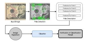
Fig. 1. Overview of the main processing stages of the banknote recognition system.
