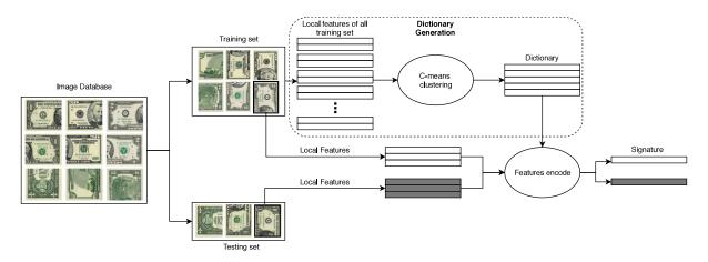
Fig. 3. Flowchart for signatures using BoVW.
