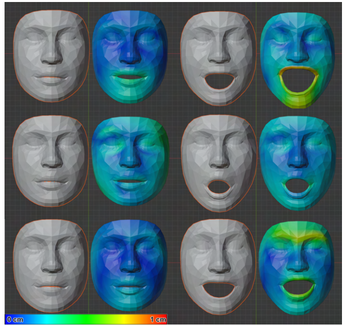
Figure 11. Blendshape adjustment error. Each vertex is painted in a colored scale, where dark blue is an error of 0 cm and bright red of 1 cm or more.
