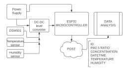
Fig. 4. System working diagram
