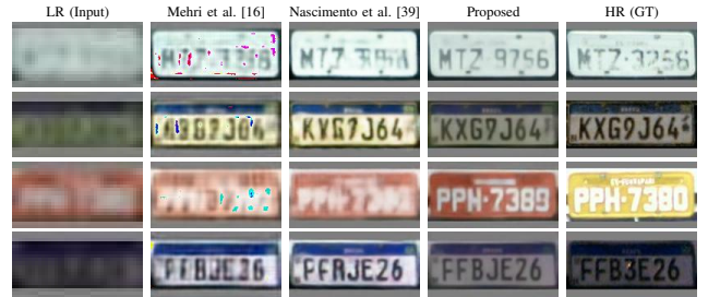
Fig. 7. Typical examples of the images generated by the proposed approach and baselines in the RodoSol-ALPR dataset [30]. GT = ground truth.
