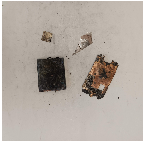
Fig. 3. Sample image of components on a white background. The components are samples of glass, PCB, battery, and metal piece, from the top right on, clockwise.
