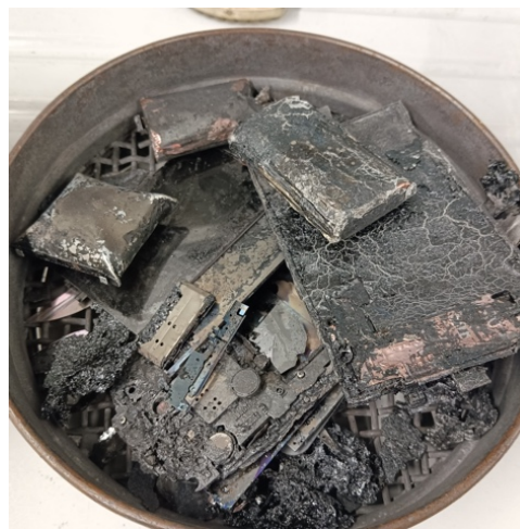
Fig. 1. Pyrolyzed smartphones for battery separation.
