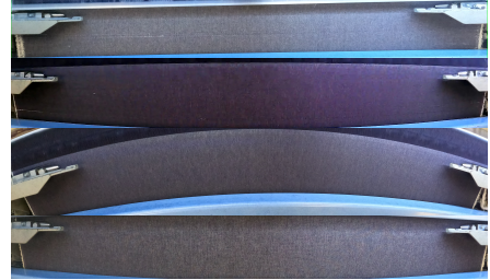
Fig. 3: Cropped image samples from the dataset. The two above are from the class “broken wefts” and the two below are “No defects”.
