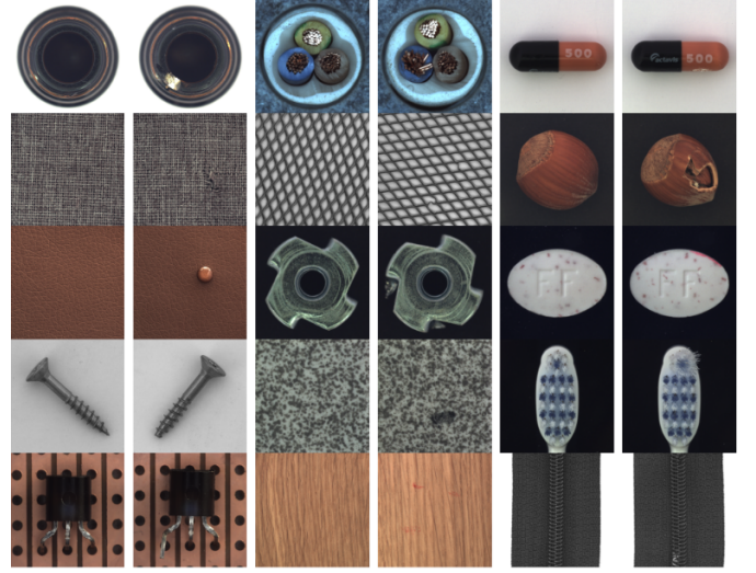
Fig. 2. MVTecAD. For each object, we have the normal and anomaly samples. Anomalies vary in each class, and can range from textures outside the acceptable standard (“grid” and “leather”, for example) to defective parts, such as the “hazelnut” shell and solders on the “transistor”.
