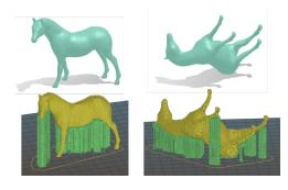
Fig. 8. Horse\_quad.obj on the initial vertex position (top-left) and after rotation (top-right). The same surface on the initial position on the print simulator (bottom-left) and after rotation (bottom-right). In yellow, the software indicates the solid that we want to print and in green the overhang supports.
