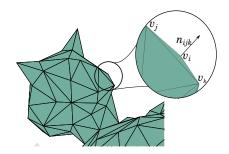
Fig. 4. In this surface, we have the vertex matrix  $\mathcal V$  and its triangle mesh matrix  $\mathcal F$ . Each triangle has three possible normal associated, but is easy to see that is all the same vector. So, we need only one of them to represent the triangle face normal vector.
