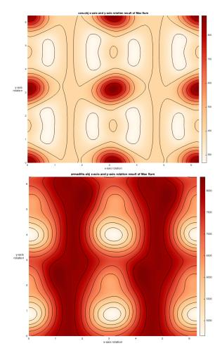
Fig. 6. These graphs represent the value (in a gradient color) of sum of max in equation 3 in a x-axis and y-axis rotation of *cow.obj* (top) and *armadillo.obj* (bottom) surface.
