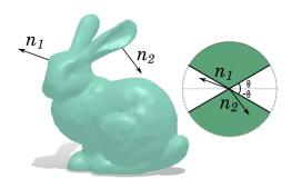
Fig. 5. This two normal  $n_1$  and  $n_2$  of the bunny surface has different angle. The normal vector  $n_1$  is in the angle parameters of the printer. The normal vector  $n_2$  is in a overhang part and will need a support to print correctly.
