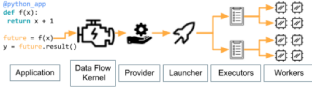
Figure 1. Simplified Parsl execution flow [Parsl Developers ].
