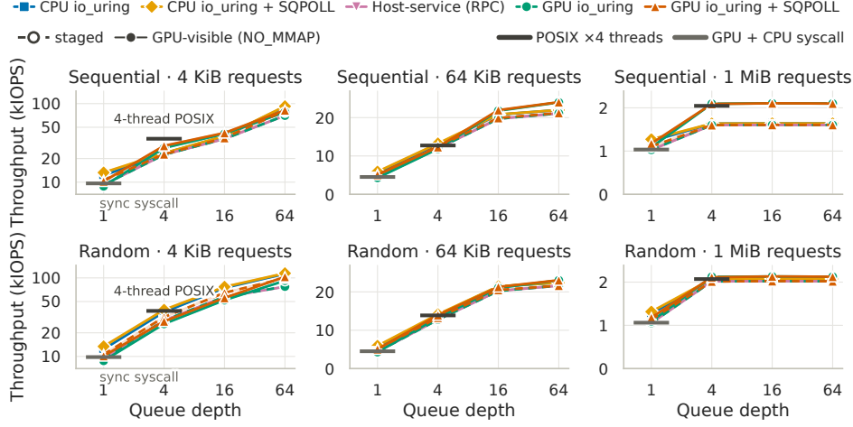
Figure 3. P100 read throughput versus queue depth and request size.
