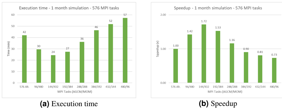
Figure 7. Performance on different distributions of 576 MPI tasks
