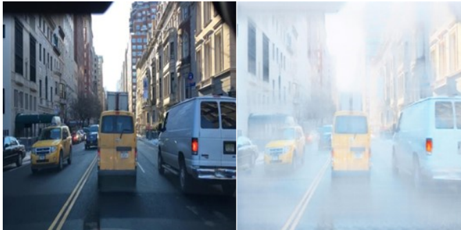
Fig. 1. On the left, we have the original image and on the right, we have the image with the application of the Foggy-Cycle-GAN algorithm transforming it into a foggy image. Source: BDD100K Dataset.
