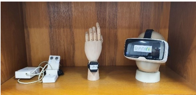
Figure 3: BRAINN_VR wearables with ultrasound and inertial sensors for controlling virtual environments.
