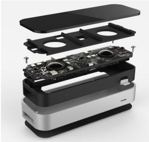
Figura 3. Leap Motion Controller [11]
