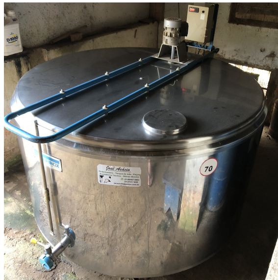
Figure 1. Cooling tank that stores milk
