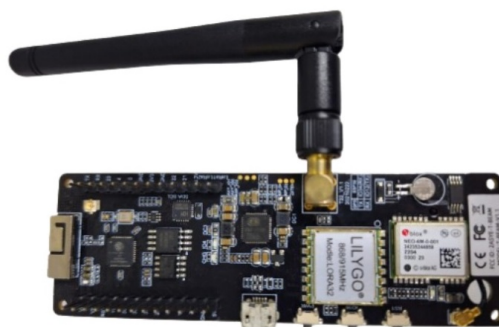
Figure 2. LILYGO module based on ESP32 and LoRa.
