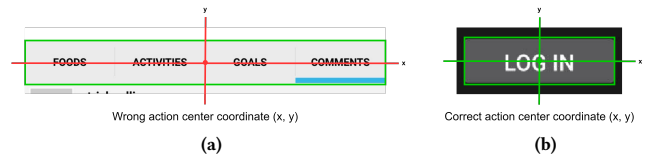
Figure 4: Example of “Multi-Tab” non-atomic widget (a) and “Text Button” atomic widget (b). Non-atomic widgets contain different atomic components, and their center coordinates (x,y) may have no effect during automated interactions (a).
