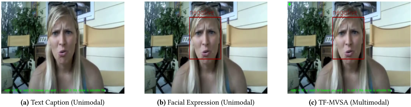
Figure 3. TF-MVSA tool demonstration over a MOSI benchmark video. In the textual modality, sentiments are color-coded in captions (green=positive, red=negative, white=neutral). For the visual modality, sentiment labels appear above face rectangles. In the multimodal version, a consensus sentiment is displayed in the top-left corner, combining both modalities' information.
