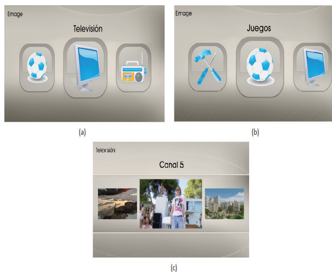
Figure 4: (a) Initial state, (b) Change when moving the head to the right., (c) Same structure in internal menus.
