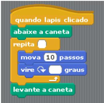
A Scratch script starting with 'quando lapis clicado' (when green flag clicked), followed by 'abaixe a caneta' (put pen down), a 'repita' (repeat) block with a blank input field, containing 'mova 10 passos' (move 10 steps) and 'vire 90 graus' (turn 90 degrees), and ending with 'levante a caneta' (put pen up). |
