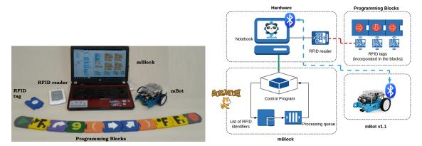
Figure 1. TaPrEC+mBot physical environment (left), system architecture (right)
