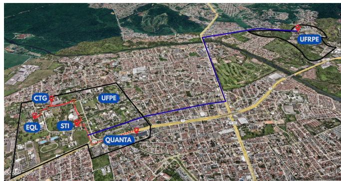
Figure 2. Current configuration of the RQN, interconnecting three main sites. At UFPE, the network links the Department of Physics (EQL laboratory at CCEN) to the Department of Electronics and Systems (CTG), while at UFRPE the connected site is the Department of Physics (LOL). Solid lines represent the optical fiber links that are already installed and operational, whereas the dashed line indicates the planned connection to QUANTA-UFPE, which is presently being implemented as part of the first expansion phase.
