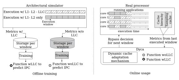
Figure 1. Diagram of the whole process of core adaptation using bypass.
