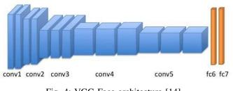
Fig. 4: VGG Face architecture [14].
