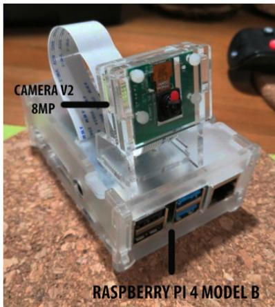
Fig. 4: Case for Raspberry and camera module.
