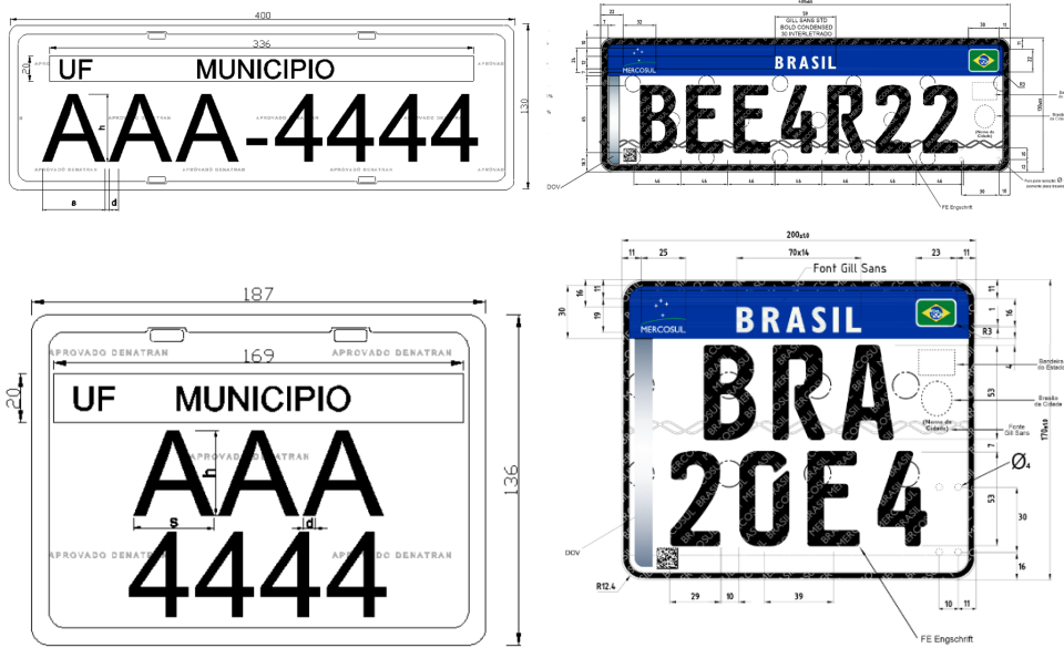
Fig. 1. License plate models in Brazil, on the left, the old model, and, on the right, the Mercosul model. Upper plates for cars and lower plates for motorcycles. Source: [4], [5].
