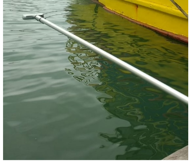
Fig. 8. Camera attached to the pole to capture images on the dikes
