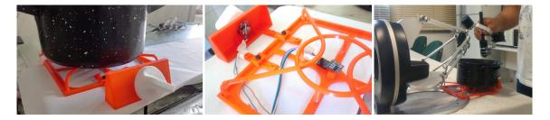
Fig. 3. Left: interactive stove knob prop, attached to potentiometer. Center: time-of-flight sensor, responsible for detecting the presence of the pot on top of the stove. Right: haptic device rendering force feedback to the user stirring the pot, virtually providing a manipulable sense of texture based on what is being cooked.
