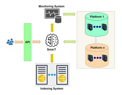
Fig. 1. SmarT architecture includes an API that interacts with users, and a central module (SmarT) responsible for choosing one of the big data platforms to run the query. SmarT makes this choice using, as input, data coming from the monitoring and indexing system, which are also part of the architecture.
