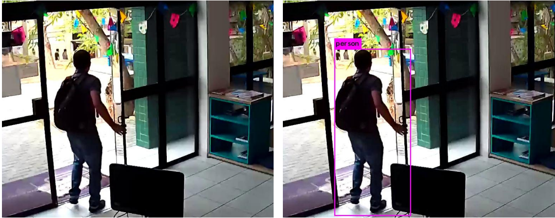
Fig. 4. The left image is a sample frame from our setup and the right one is the same frame with a bounding box indicating a detected person with a given confidence level (near the top-left corner of the bounding box).
