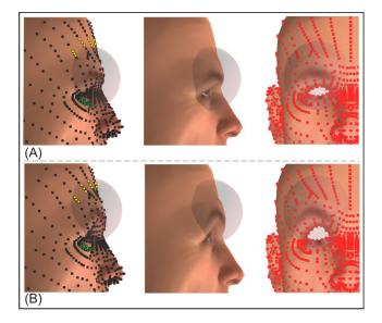
Figure 10. Moving influence zones. (A) Yellow points are initially outside the influence zone and green inside. (B) After the translation, the yellow points are inside and the greens are outside the sphere.
