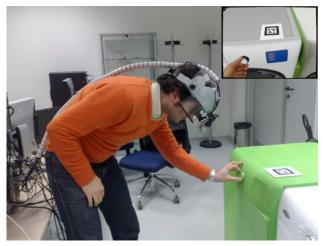
Figure 3. Virtual Prototype of a washing machine implemented using Augmented Reality technologies
