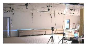
Figure 5. Motion capture area used for the study on stepping. Cameras are fixed to the wall, the ceiling or on tripods. On the ground one can see a video-projected calibrated pattern to guarantee the correct display of targets [15].
