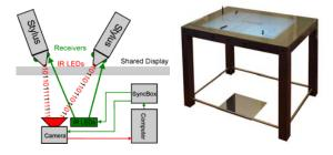
Figure 3. Principle setup of InfrActables and its realization
