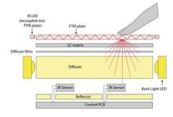
Figure 7. IR-sensors in the LC-screen
