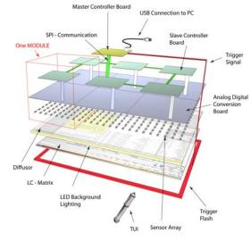
Figure 5. Principle setup of the MightyTrace
