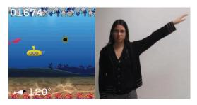
Figure 8. User's body is tracked and the patient is required to practice a specific movement of interest in his/her treatment. Then the movement is evaluated by the system and a correction suggested when needed.
