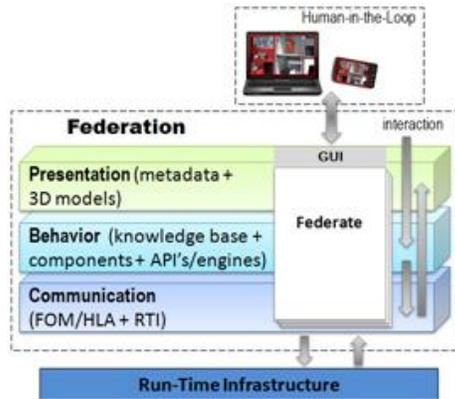
Figure 7. Overview of layer architecture.
