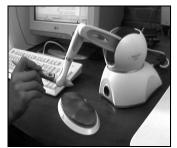
Figure 1. Phantom Omni haptic device used in VR systems and in the Bone Marrow Harvest simulator.
