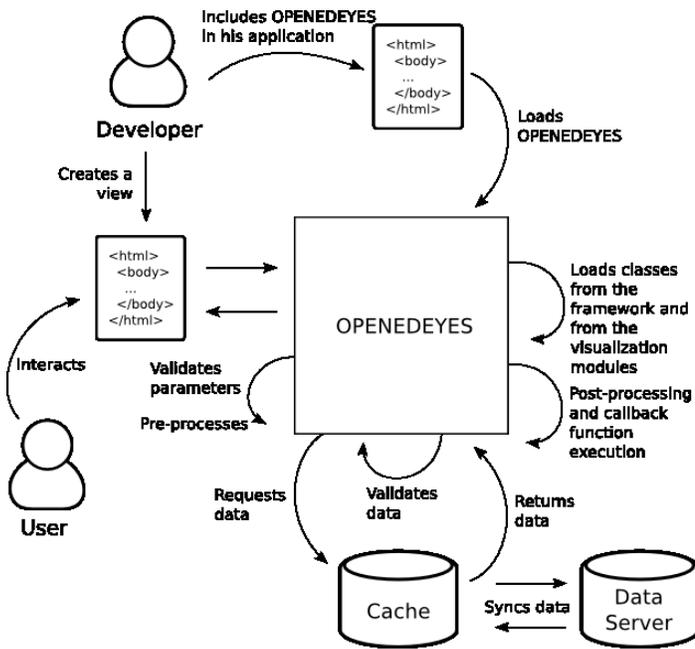
Fig. 2. Global execution flow of OPENEDEYES
