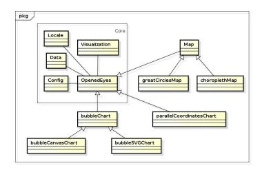
Fig. 3. Simplified OPENEDEYES class diagram
