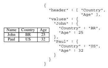
Fig. 16. A typical data table and its corresponding OPENEDEYES JSON structure
