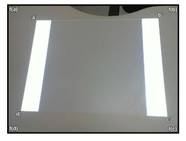
Fig. 10. Correspondent points used to align the camera-projector system.
