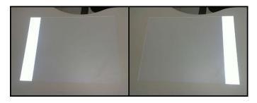
Fig. 9. Structured lights projected in sequence so the alignment can be calculated.
