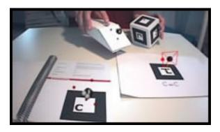
Fig. 2. Augmented Chemistry in use. The user holds a claw with the right hand and a cube for orientation with the left hand. On the bottom left corner there is a catalogue of periodic elements and over the marker on the right there is the molecule assembled by the student.
