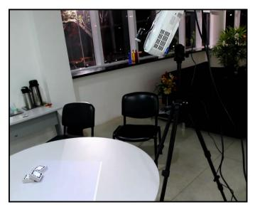
Fig. 11. Camera-projector system setup, using a tripod. The projector illuminates the table where the children can use the system.
