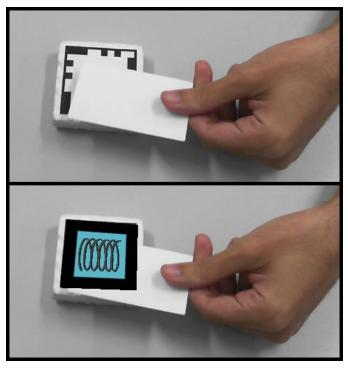
Fig. 8. The original image, on the top, shows that most of the marker is occluded. Even though, in the bottom it is possible to see that the block is tracked and the augmented reality content is rendered over it.
