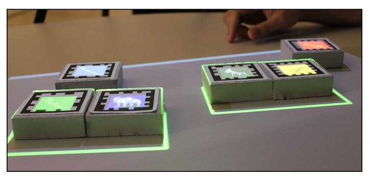
Fig. 12. The information is projected only on the blocks empty area. The green line around some blocks denotes to positive feedback when the activity is executed correctly.
