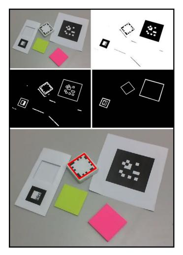
Fig. 6. The original frame captured by the camera appears on the top left of the image and on the top right there is the result from the segmentation process; the row in the middle shows every line extracted by the Canny and only the quadrilaterals that could be markers; in the end, only the proposed marker is selected.
