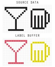
Fig. 11. Labeling example (with correct label equivalence).
