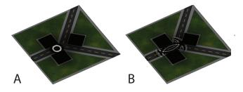
**Fig. 9:** Test scene geometry and the wave propagation effect evolving through time (from A to B). Parts (A) and (B) omit buildings to help in visualizing wave reection.
