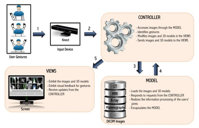
Fig. 4: Architecture of the gesture-controlled system. The user performs a gesture that is identified by the camera of the *Kinect* input device. Through the CONTROLLER, the VIEWS of the MODEL are modified according to the user selected functionalities.
