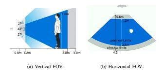
Fig. 7: In (a) and (b), the *Kinect* vertical and horizontal FOV in default range, respectively [31].
