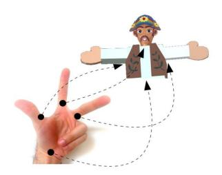
Figure 8. Association scheme between hand and puppet joints.
