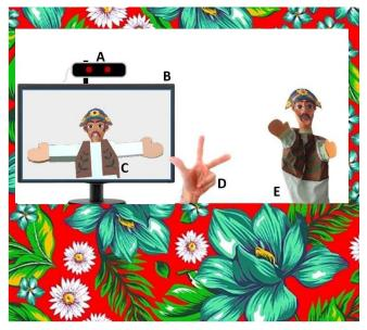
**Figure 14.** Tent's layout: A) Leap Motion; B) LCD monitor; C) Virtual Puppet; D) Virtual Puppet handler's hands; E) Real Puppet.
