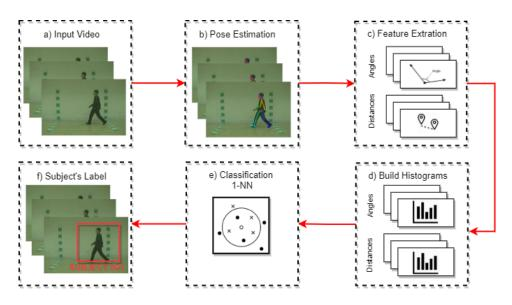
Figure 4. Block diagram of the proposed method for gait recognition using 2D poses.
