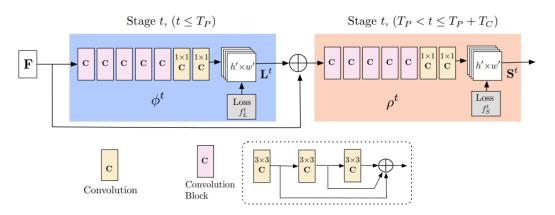
Figure 2. OpenPose CNN architecture [Cao et al. 2018].
