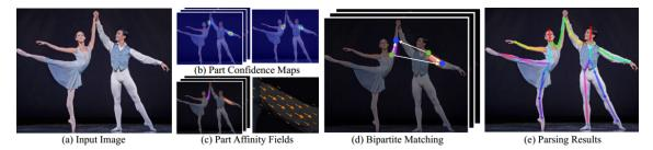
Figure 1. Pipeline of the OpenPose method [Cao et al. 2018].
