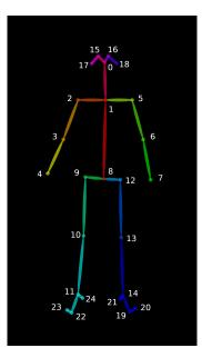
Figure 5. Pose output format of BODY\_25 [Cao et al. 2018].
